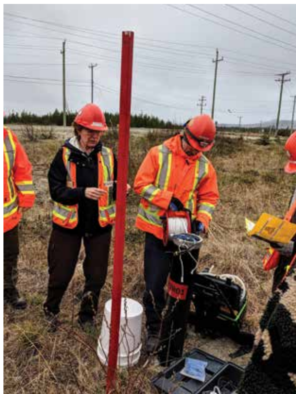
Staff members from the Eleonore mine demonstrate groundwater sampling at the mine site, June 2019.
